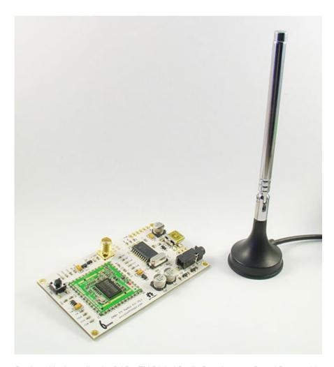
Designed in Australia, the DAB+ FM Digital Radio Development Board Pro provides a platform for developing and evaluating DAB+, SlideShow and FM receiver. The board contains a Keystone T2\_L4A\_8650C DAB/FM module and a Microchip PIC18F14K50 microcontroller. The T2\_L4A\_8650C module is an ultra low power DAB/FM receiver module with the following features:
